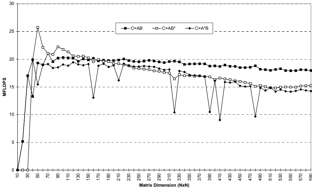
Figure 4-13: Performance of the low-level routines for the SPARCstation 4 (SPARC 110MHz) 32 MB (average of 3 tests)
